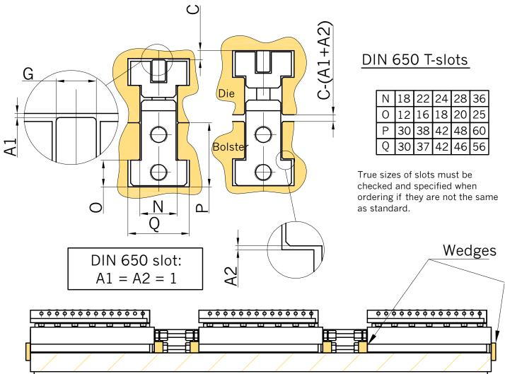
LSGH clamps must be stopped in translation in the slot (and not fixed), by mean of wedges. When coupling 2 bars or more, they must be blocked individually, so that no strain is applied on piping.
