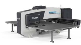
Single-head punch press that can punch, bend, tap and form all on a single machine
