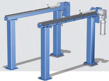
The Motorized Bolster Extensions (MBE) combine the functionality of bolster extensions and push-pull system into one integrated unit. MBEs support the die outside of the press and transfer the die in and out of the press. The die can be loaded with either an overhead crane or a fork-truck. MBEs also allow easy access to the side of the press. Since they are
